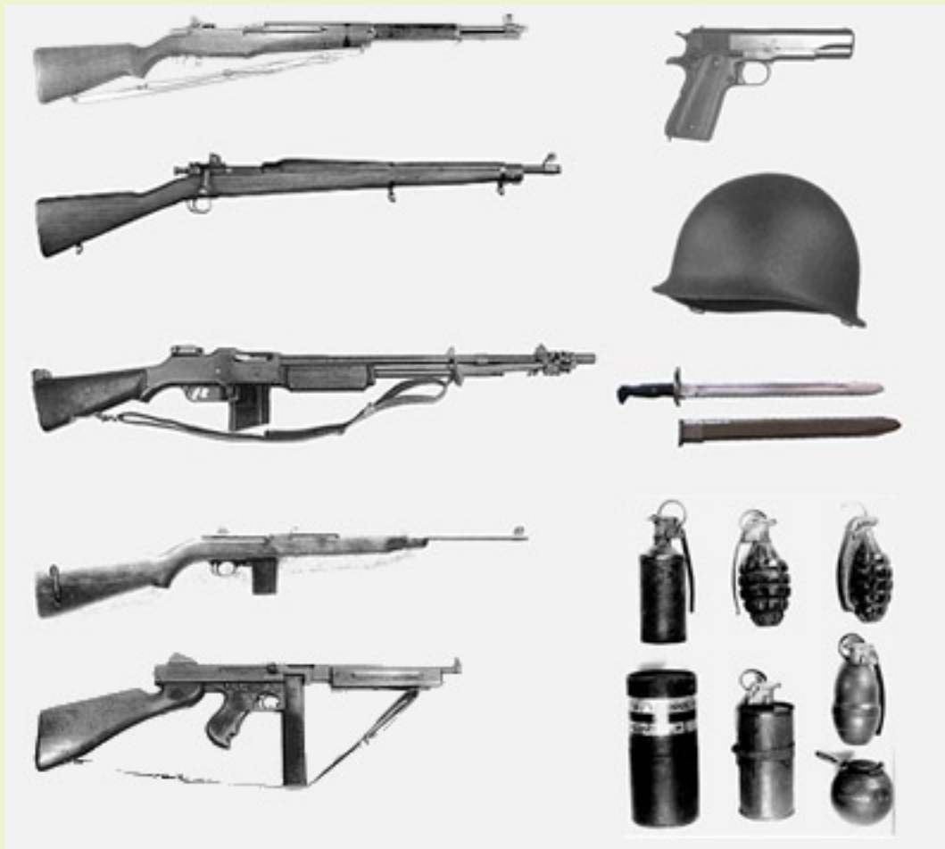
Standard US Infantry Weapons and Armor (left column: M1 Garand, M1903 Springfield, M1918 Browning Automatic Rifle, M1 Carbine, M1928 Thompson Submachine Gun; right column: M1911 Colt .45 Pistol, M1 Steel Helmet, M1 Bayonet, Assorted grenades)
