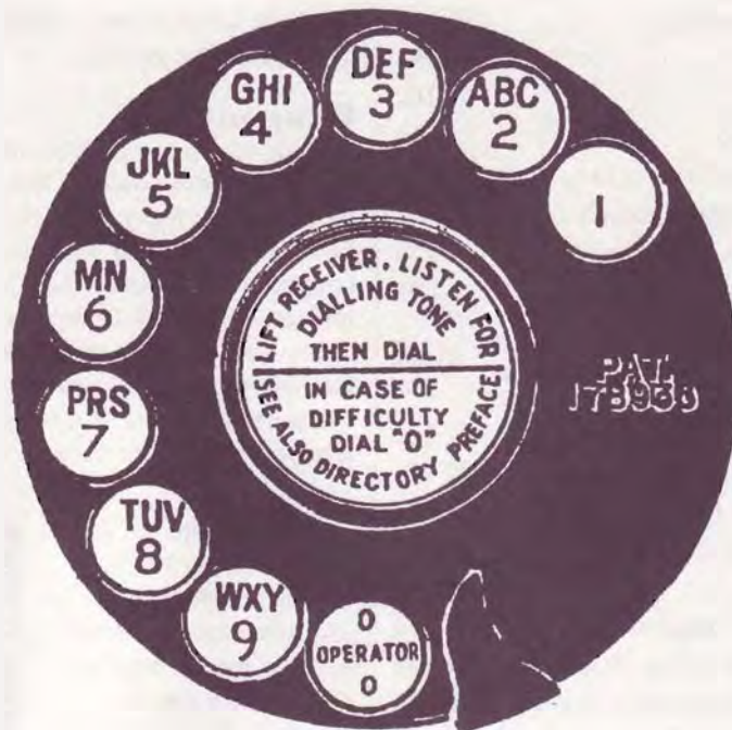
The standard auto telephone dial, London type, of 1925.
